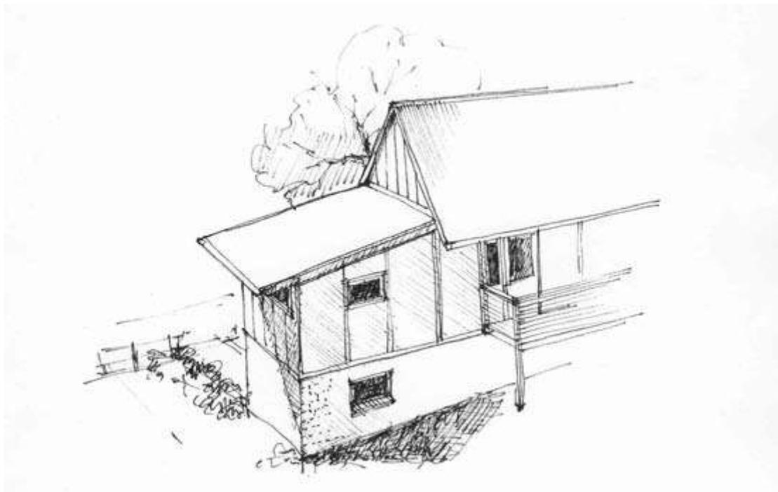
**Window awnings:** fixed window awnings are increasingly being used to provide precise shading. There are many examples of fixed awnings from early buildings that can be adopted or modified.
