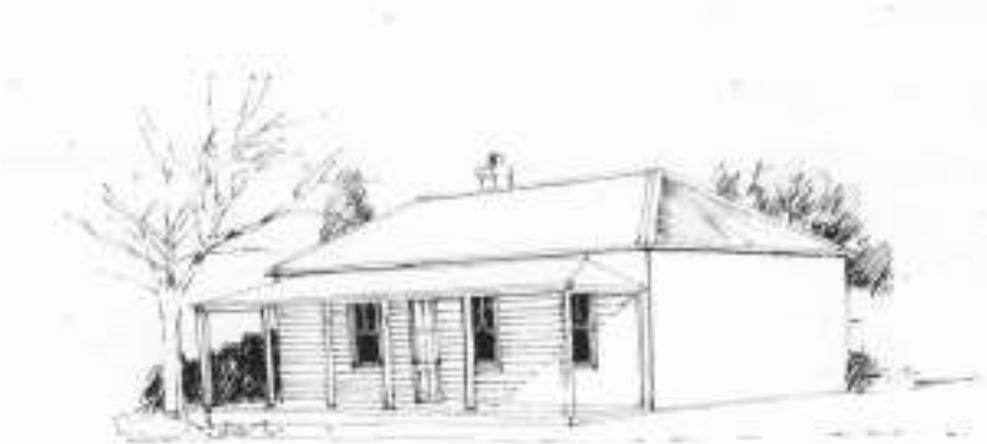
2. Classic weatherboard cottage with hipped roof and lower pitched hipped verandah to the street frontage. Vertically proportioned windows, slender hardwood posts with simple arched detailing. Corrugated steel roof. Ceiling height usually 3 metres.
