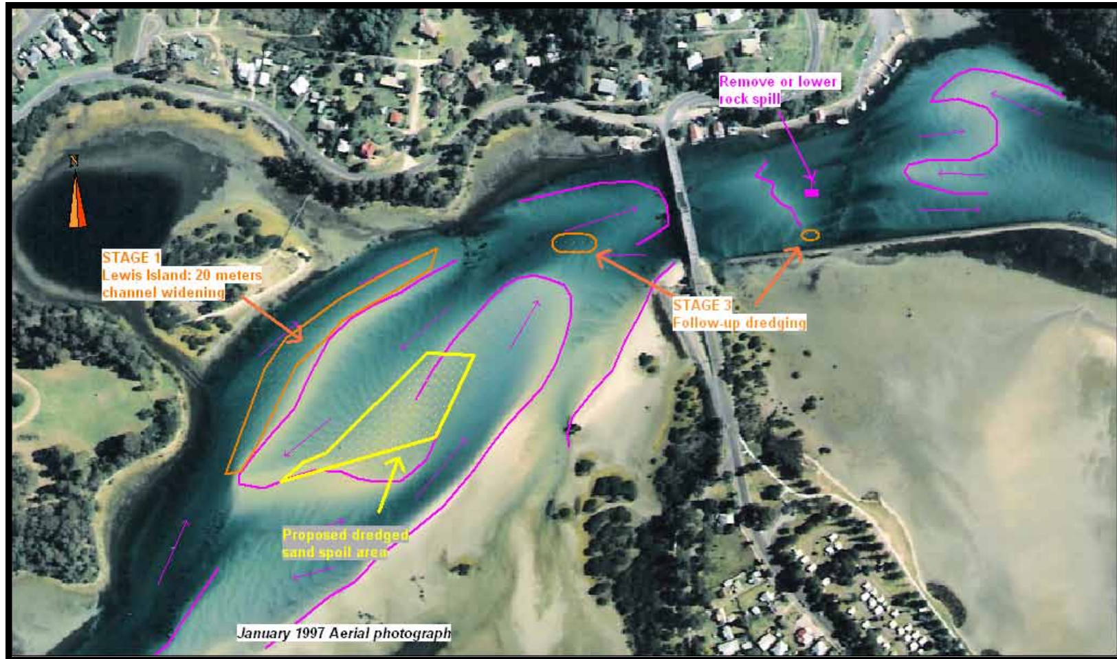
Figure 1b Localities of proposed mid-channel works around highway bridge (Jan 1997 aerial photo base).
