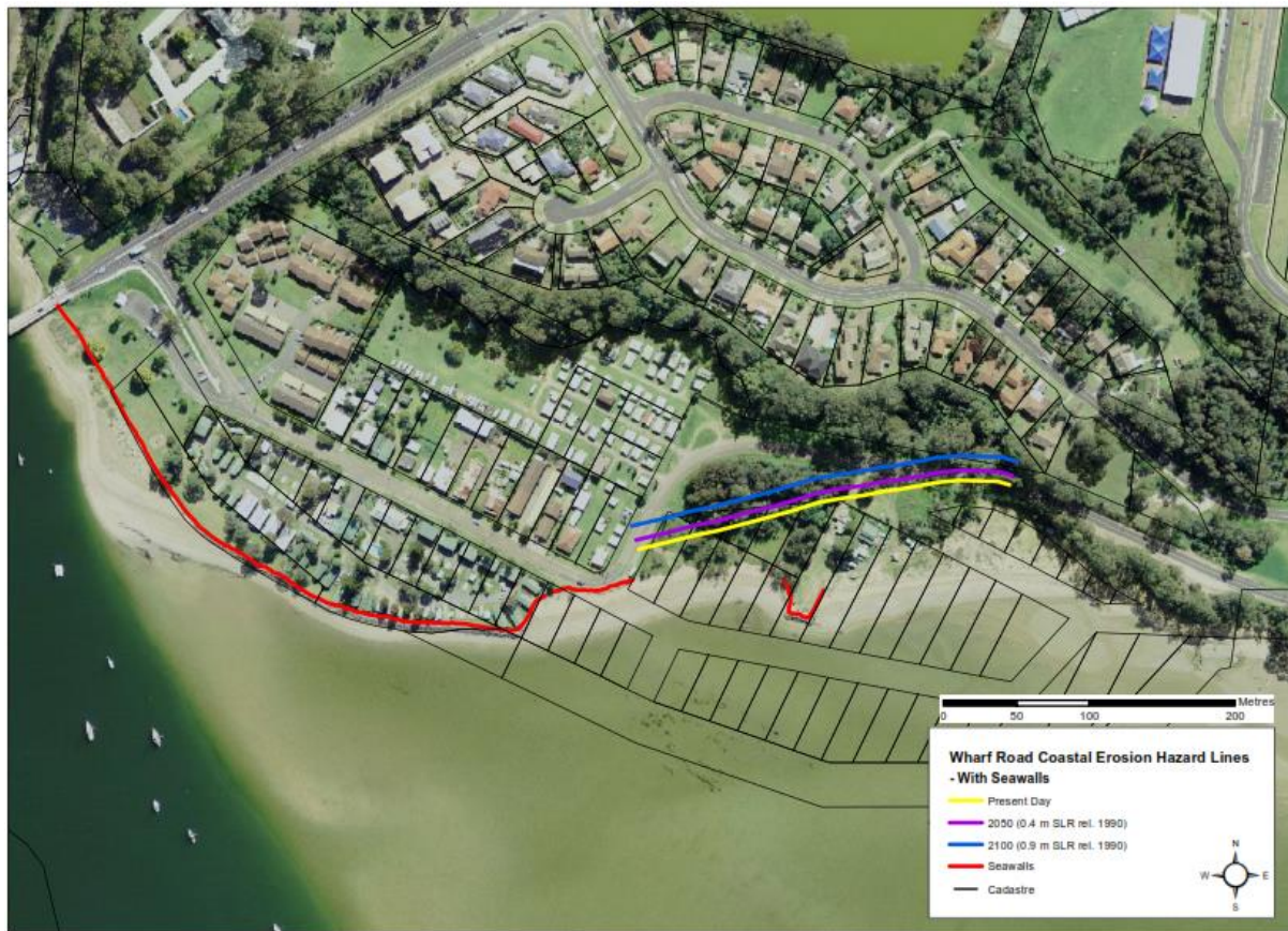
Figure 5: Extract from WRL 2012 showing coastal erosion
