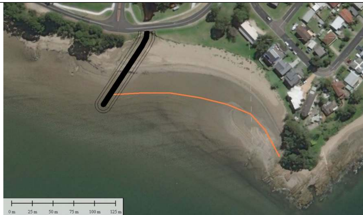
Figure 1. Indicative alignment of a culvert extension/groyne structure (black) at Macleod's beach with anticipated shoreline response (orange)
