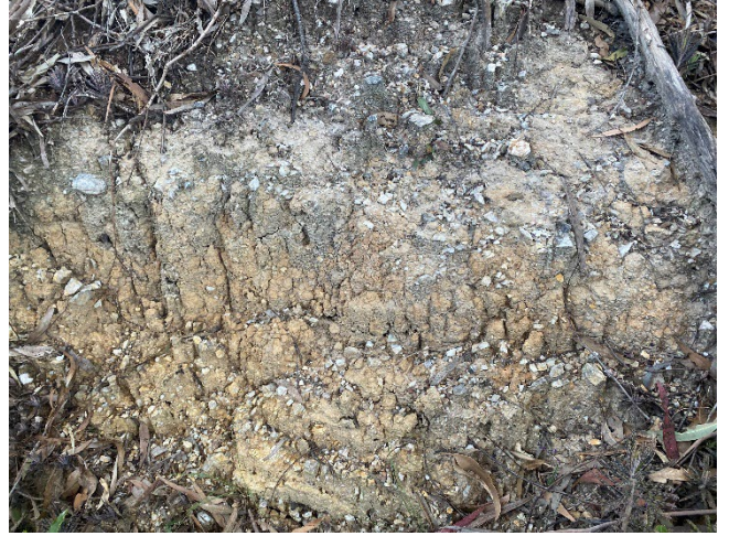
Photo 19: Area of exposure along eastern side of Bermagui Service Road showing mixed deposit of white quartz, leaf litter and yellow-brown sandy clay
