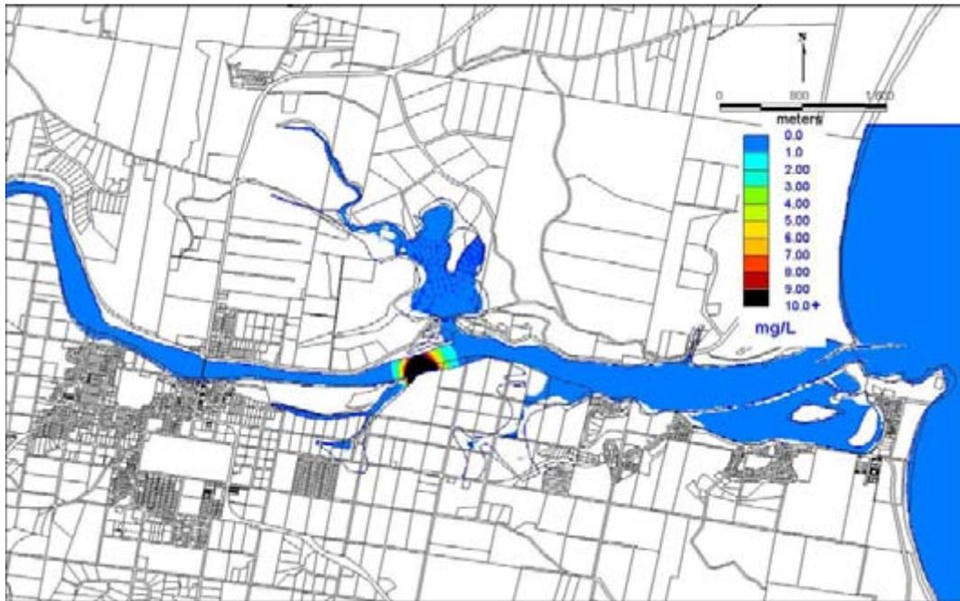
Figure 4.18: Dispersal of Dye after 1 hour, Scenario 2.
