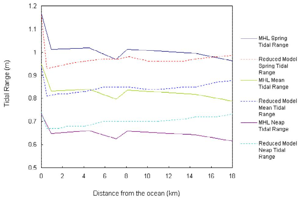
Figure 2.22: Comparison of measured (MHL) and Reduced Model tidal ranges with MHL tide driven simulation.
