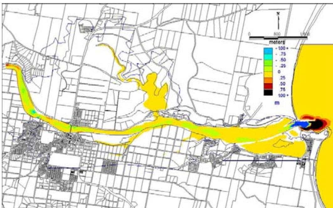
Figure 3.6: Bed change in the lower estuary for 1 Year Flood with mean tide action. (Note black represents deposits greater than 1 metre high, dark blue erosion of more than 1 metre.)
