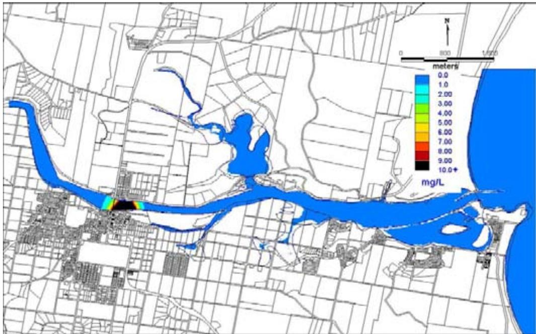
Figure 4.22: Dispersal of Dye after 1 hour, Scenario 3.
