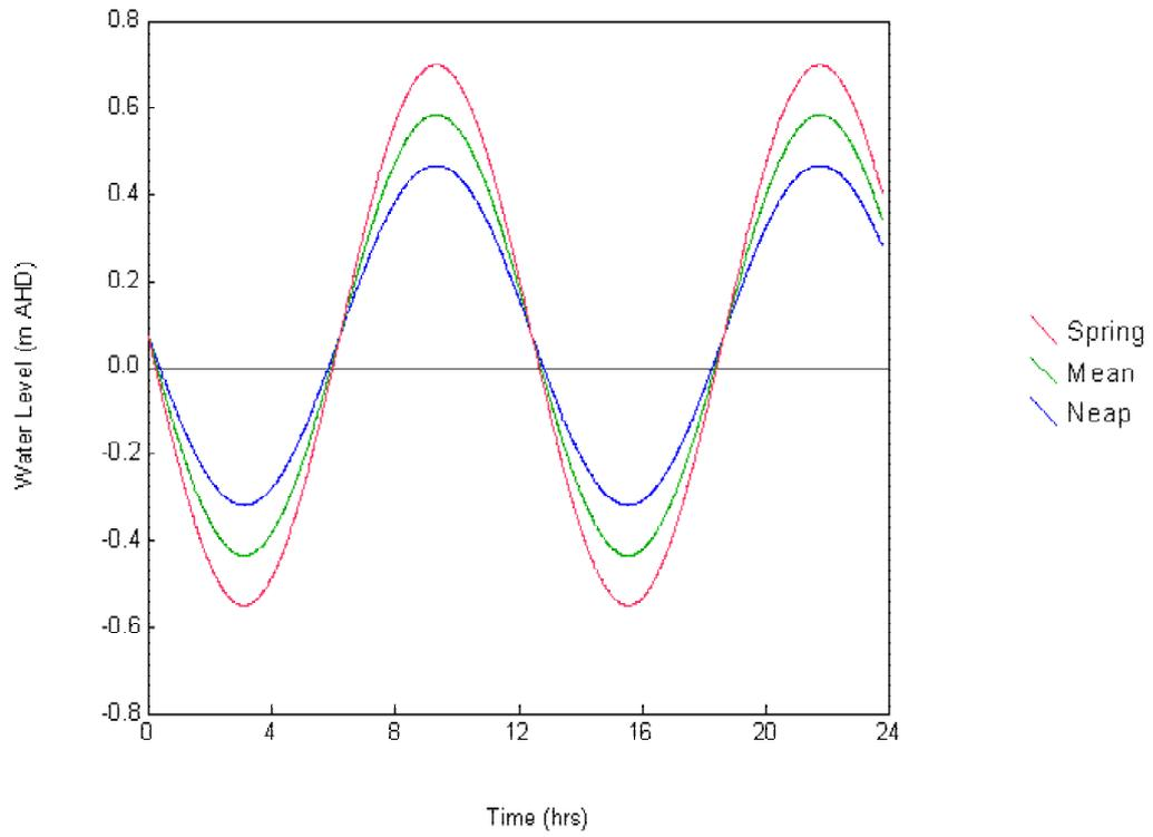
Figure 2.12: Derived Jervis Bay tidal elevations.
