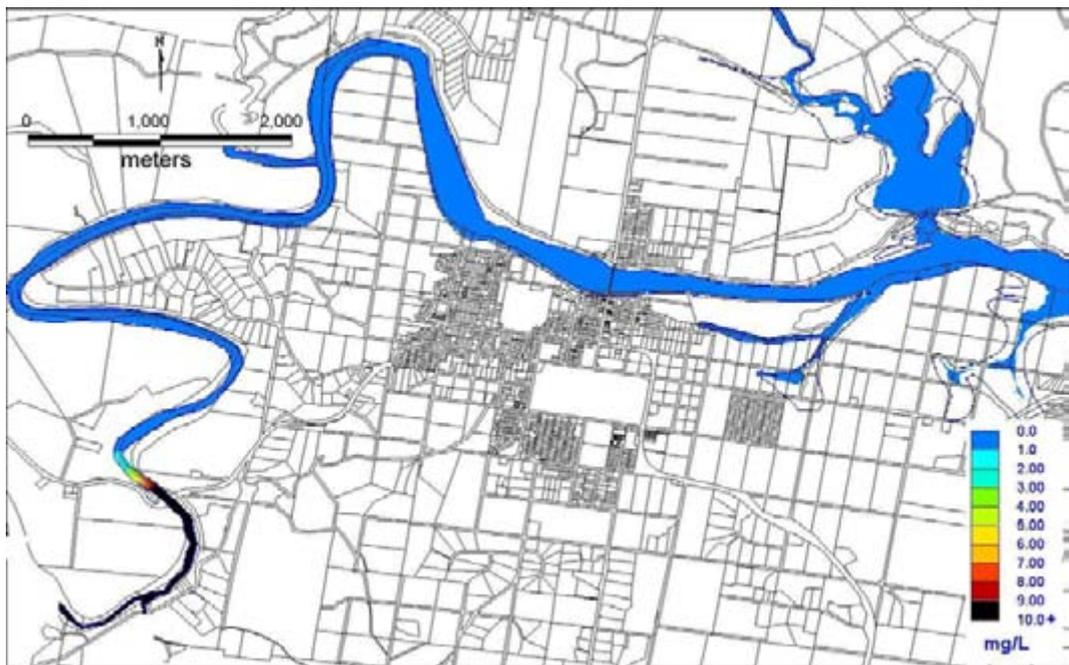
Figure 4.26: Dispersal of Dye after 6 hours, Scenario 4.
