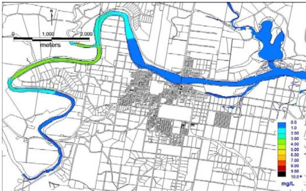
Figure 4.29: Dispersal of Dye at the end of the simulation, Scenario 4.
