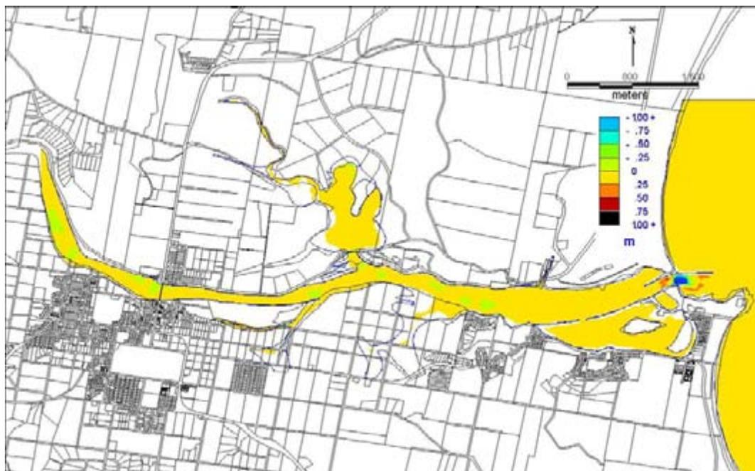
Figure 3.5: Bed change in the lower estuary for median inflow with mean tide action. Bed depth changes recorded at 25 cm intervals. (Note dark blue represents erosion of more than 1 metre.)
