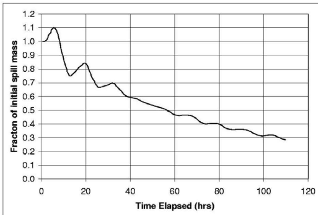
Figure 4.17: Dye Flushing from the Moruya Estuary, Scenario 2.
