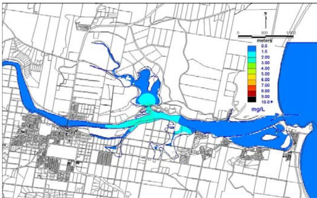
Figure 4.20: Dispersal of Dye after 12 hours, Scenario 2.
