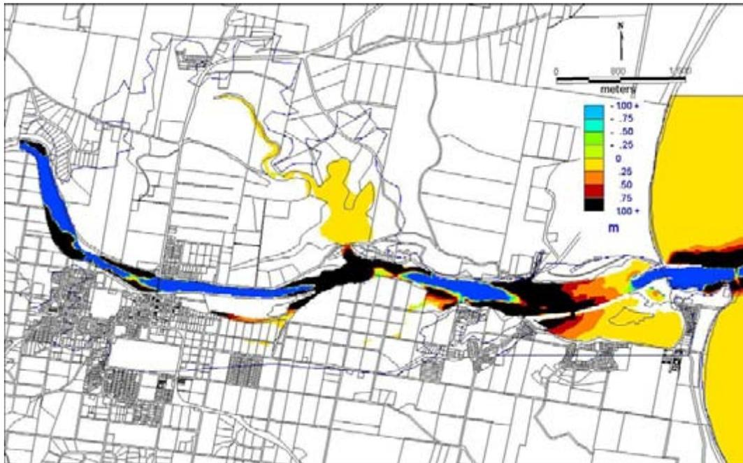
Figure 3.8: Bed change in the lower estuary for 20 Year Flood with mean tide action. (Note black represents deposits greater than 1 metre high, dark blue erosion of more than 1 metre.)
