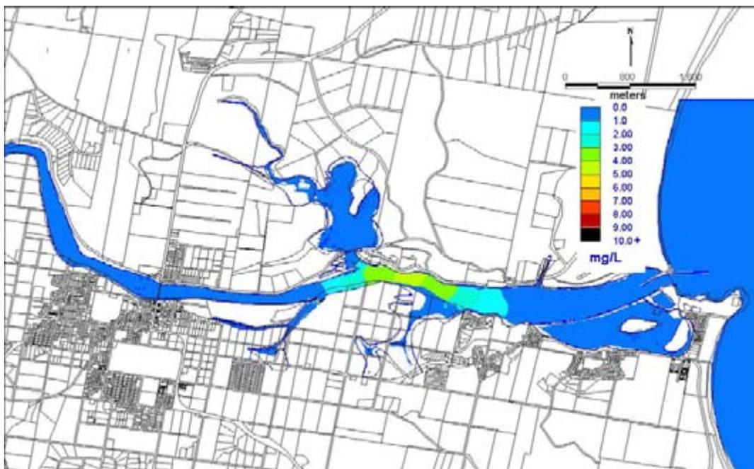
Figure 4.23: Dispersal of Dye after 6 hours, Scenario 3.
