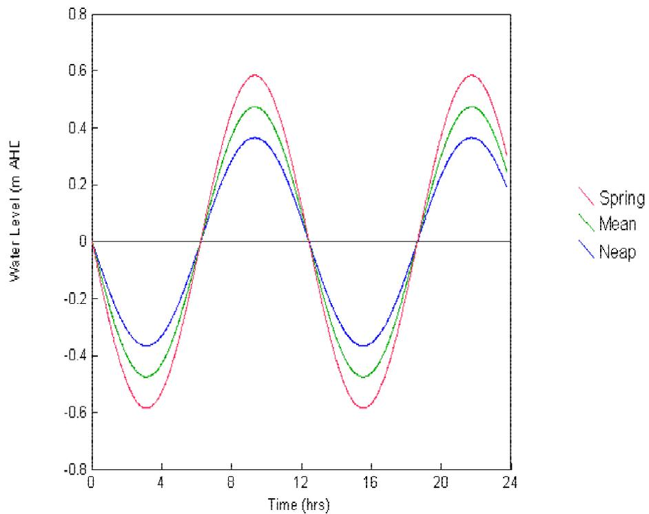
Figure 2.13: MHL data derived tidal elevations.
