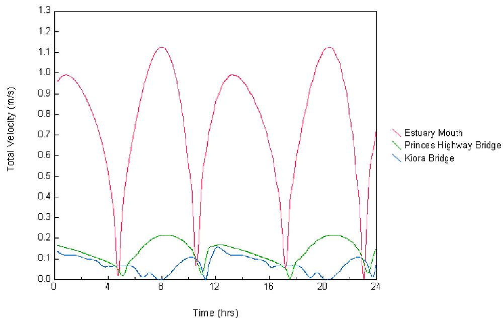
Figure 2.24: Reduced Model predicted tidal velocities in the lower, mid and upper estuary, MHL tide driven simulation.
