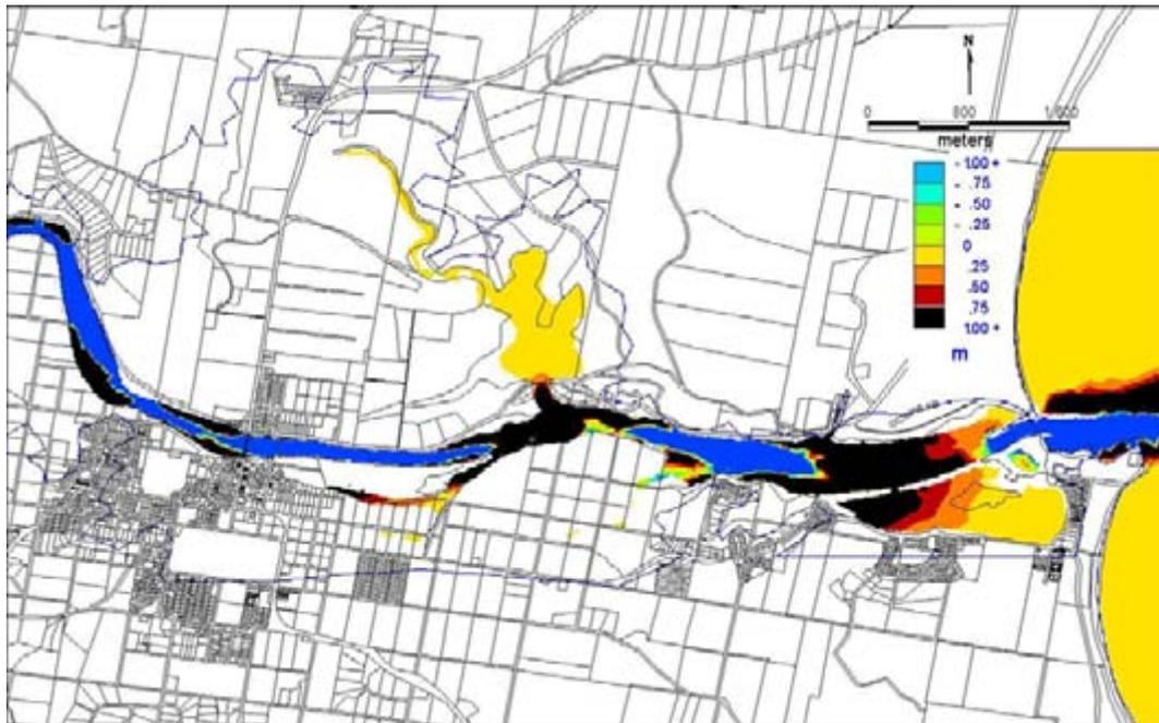
Figure 3.9: Bed change in the lower estuary for 50 Year Flood with mean tide action. (Note black represents deposits greater than 1 metre high, dark blue erosion of more than 1 metre.)
