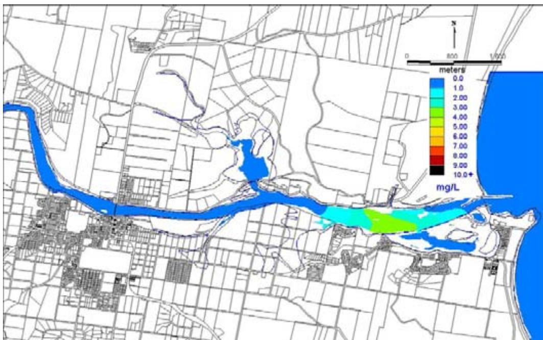
Figure 4.19: Dispersal of Dye after 6 hours, Scenario 2.
