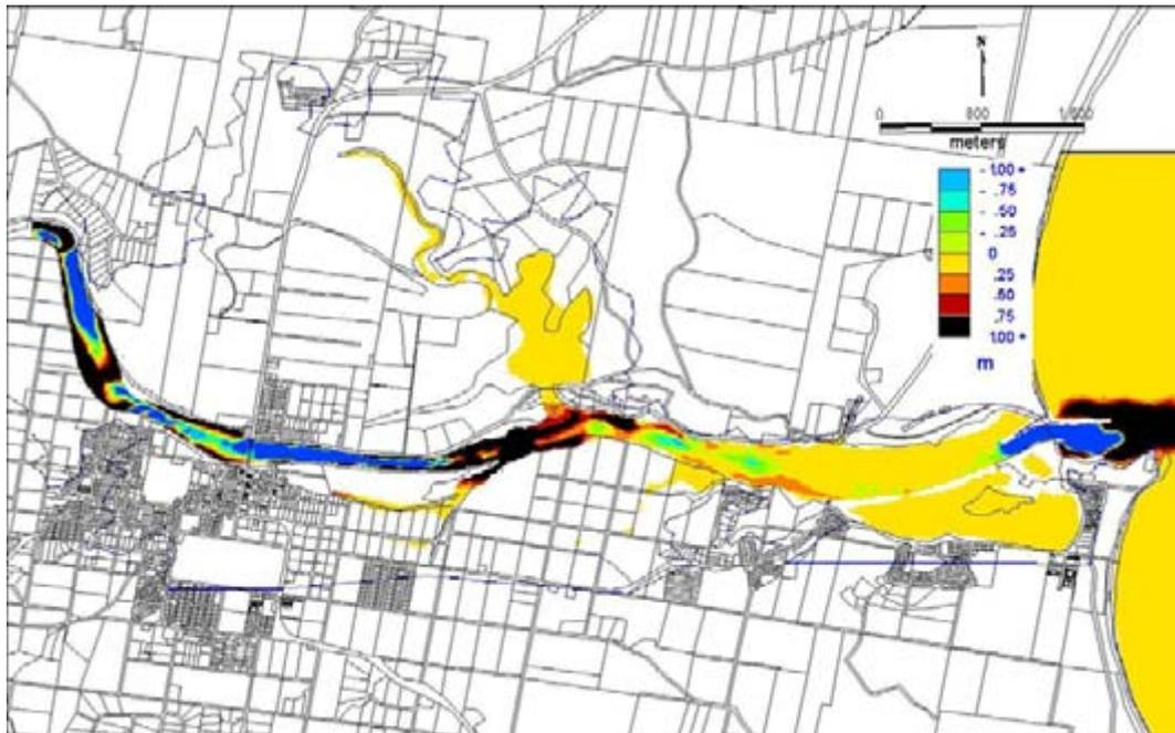
Figure 3.7: Bed change in the lower estuary for 5 Year Flood with mean tide action. (Note black represents deposits greater than 1 metre high, dark blue erosion of more than 1 metre.)
