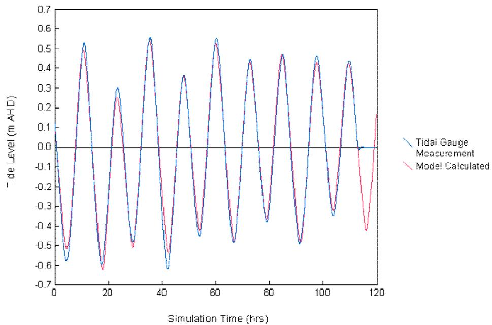
Figure 2.11: Princes Highway Tidal Gauge reduced model calibration results.
