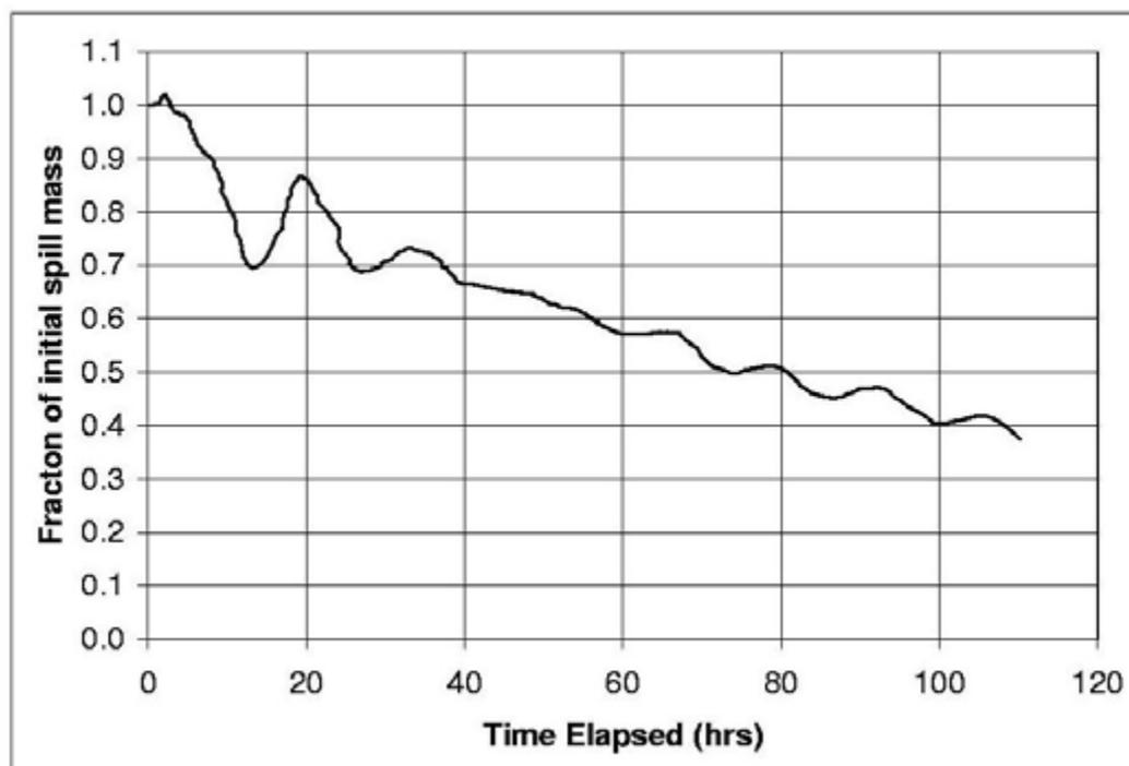
Figure 4.21: Dye Flushing from the Moruya Estuary, Scenario 3.
