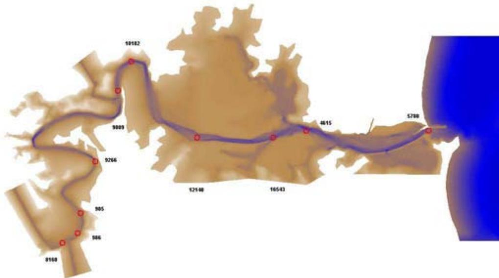
Figure 2.14: Model hydrodynamics data output points for the Full Model.
