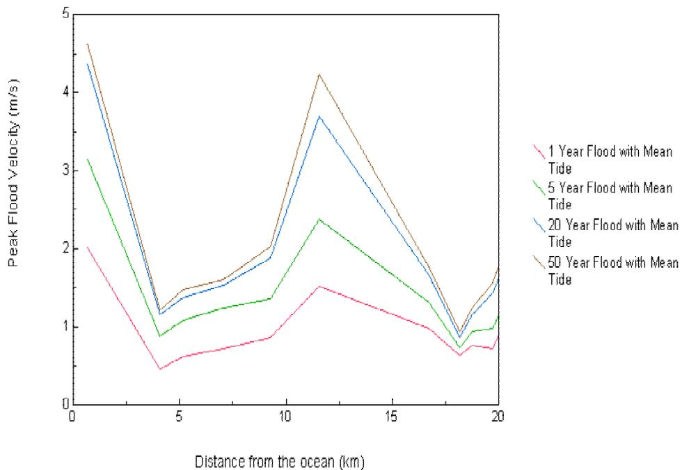
Figure 2.21: Model predicted peak flood velocity along the estuary.
