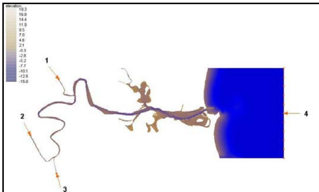
Figure 2.7: Moruya Estuary reduced finite element mesh model. Flow boundaries 1) model inflow from Mogendoura Creek, 2) model inflow from the Deua River, 3) combined model inflow from Wamban and Candoin Creeks, 4) model inflow from the ocean.
