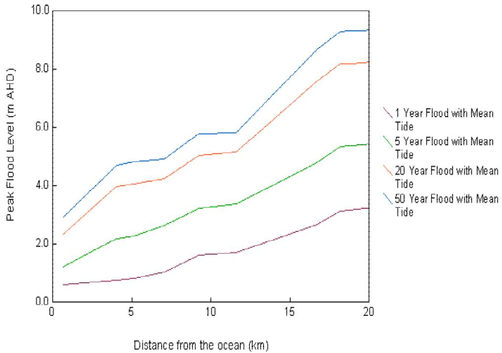
Figure 2.20: Full Model predicted peak flood levels.
