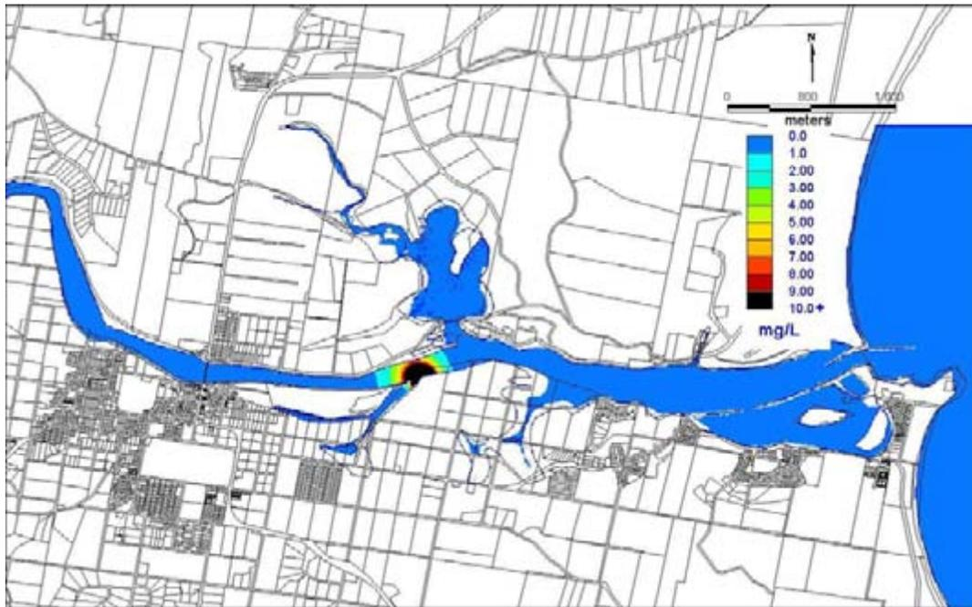
Figure 4.14: Dispersal of Dye after 1 hour, Scenario 1.
