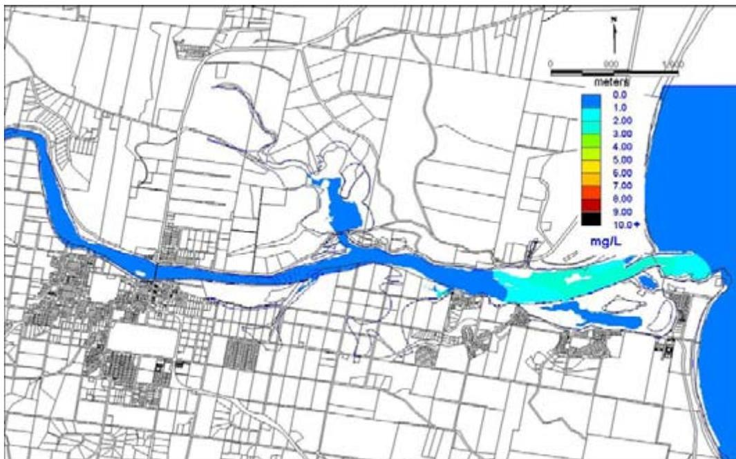
Figure 4.15: Dispersal of Dye after 6 hours, Scenario 1.
