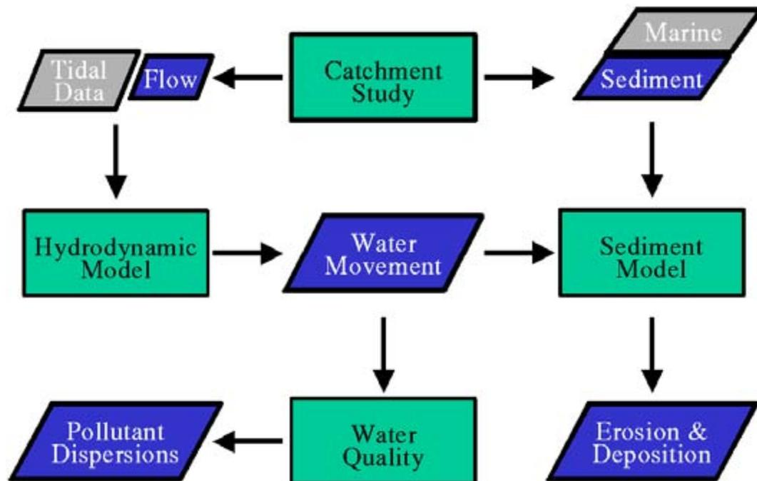
Figure 1.11: Hydrodynamics, water quality and sediment transport modelling process.
