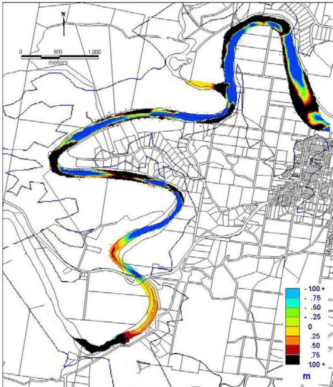
Figure 3.10: Bed change in the upper & mid-estuary for 5 Year Flood with mean tide action. (Note black represents deposits greater than 1 metre high, dark blue erosion of more than 1 metre.)
