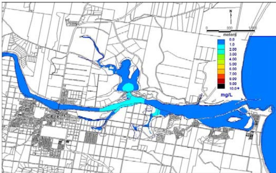
Figure 4.16: Dispersal of Dye after 12 hours, Scenario 1.
