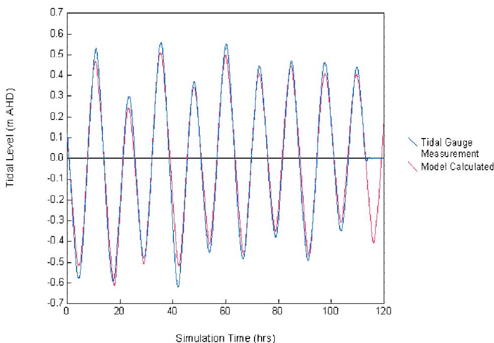
Figure 2.9: Full model calibration results for Princes Highway Tidal Gauge.
