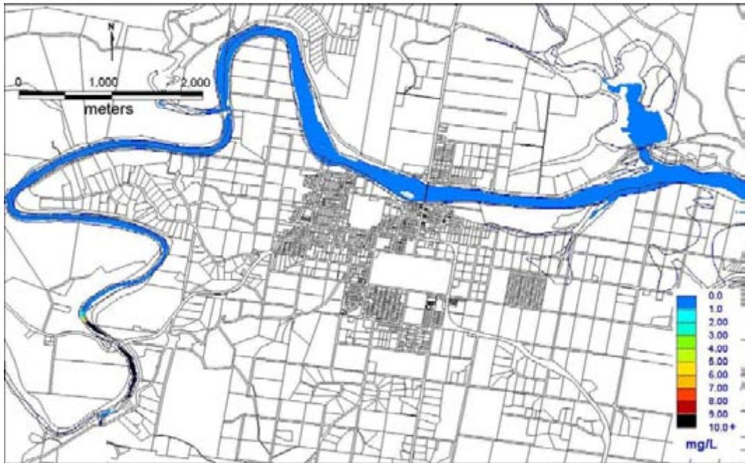
Figure 4.25: Dispersal of Dye after 1 hour, Scenario 4.
