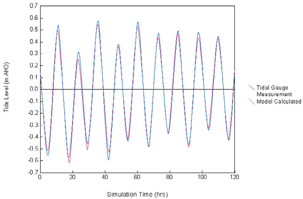
Figure 2.10: Moruya Hospital Tidal Gauge reduced model calibration results.
