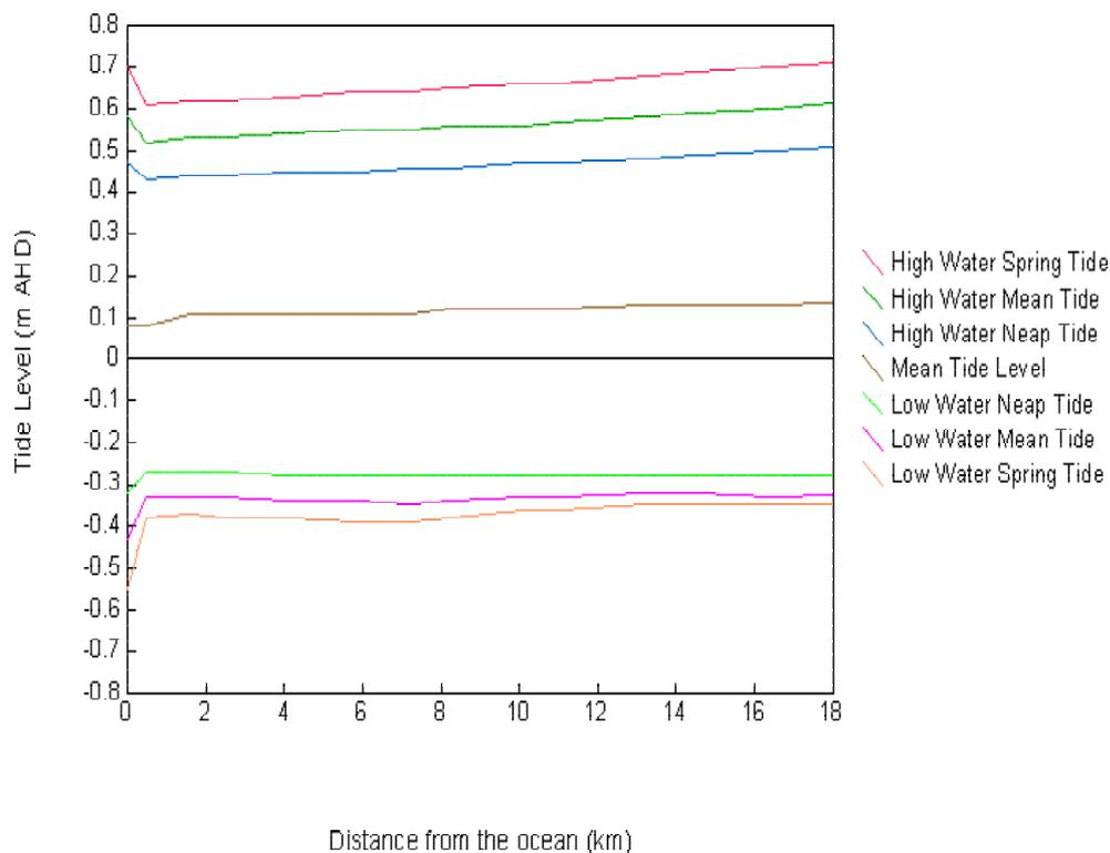
Figure 2.18: Reduced Model predicted tidal levels for Jervis Bay tides with median inflow.
