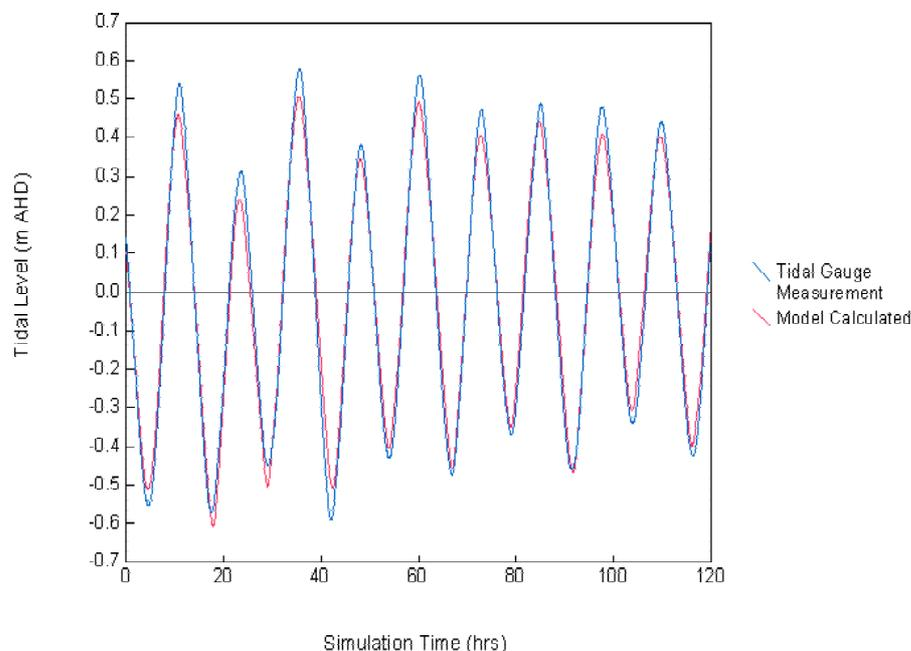
Figure 2.8: Moruya Hospital Tidal Gauge full model calibration results.
