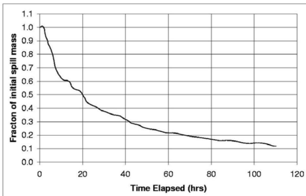
Figure 4.13: Dye Flushing from the Moruya Estuary, Scenario 1.
