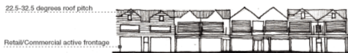
Figure 7: Indicative Commercial Street Frontage and Roof Form
