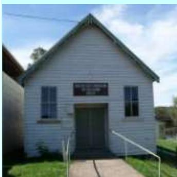
The Mechanics Institute displays a number of key characteristics of Nelligen's historic buildings including weatherboard walls, symmetrical façade, steeply pitched corrugated iron roof and vertically proportioned timber windows.
