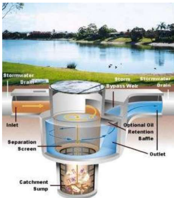
Typical cross-section of the CDS Gross Pollutant Trap
