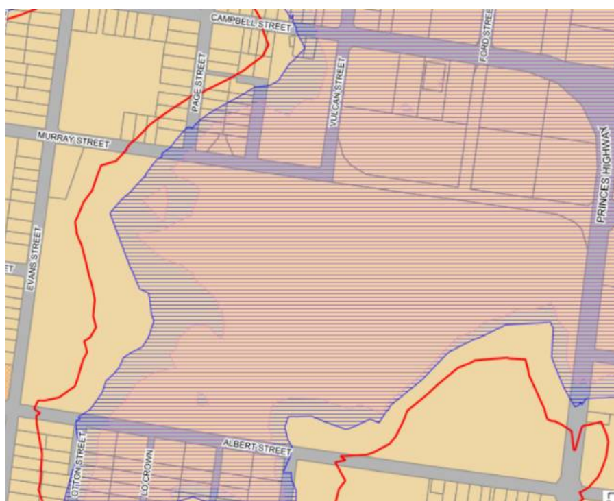
Figure 4 - Adopted flood studies showing the extent of 1 in 20 year (red hatch), 1 in 100 year (blue hatch overlay) and red line indicating probable maximum ever flood level
