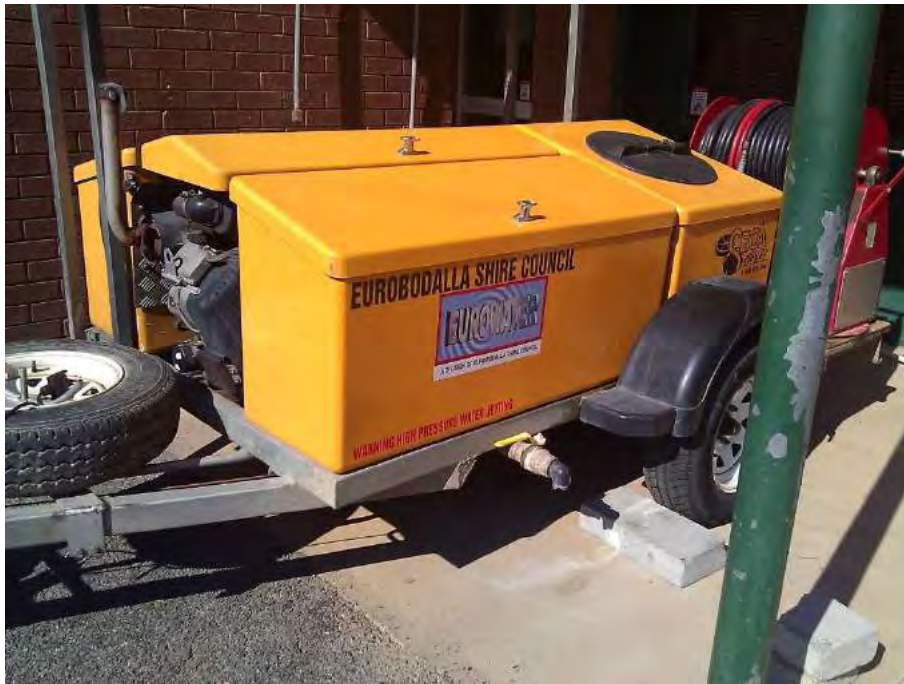
Figure 6 - 2: Water Jetter Stored at Batemans Bay STP
