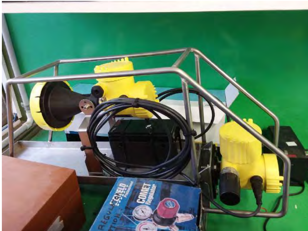
Figure 12 - 3: Portable Overflow Measurement Device Used in Batemans Bay STP
