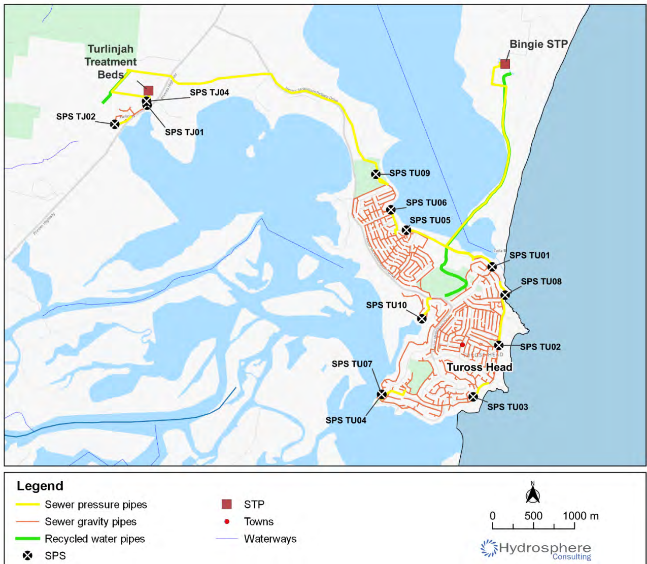
Figure 13: Tuross Head sewerage system
