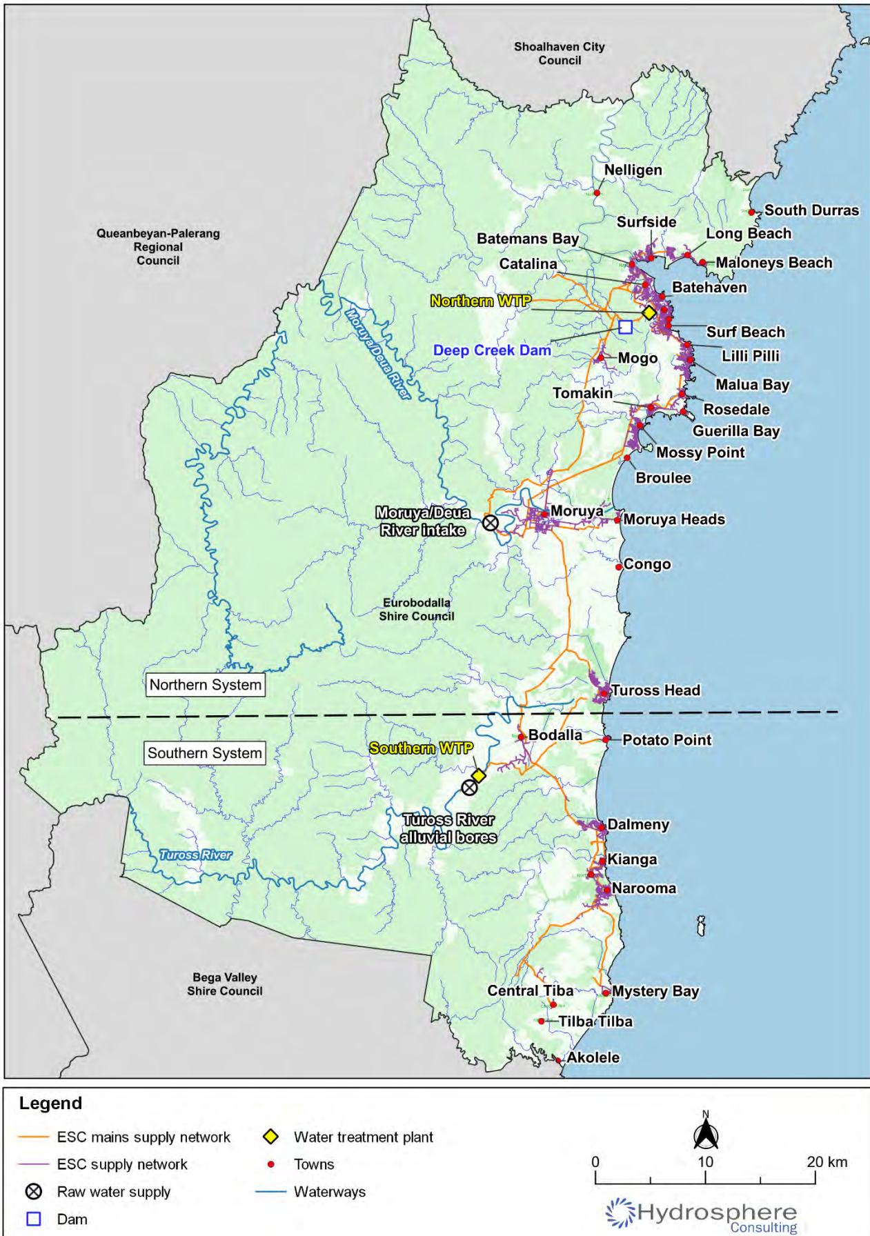
Figure 8: Eurobodalla water supply system - existing
