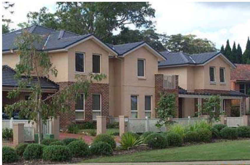
Landscaping and fence design has not blocked sight lines or created concealment spaces.
