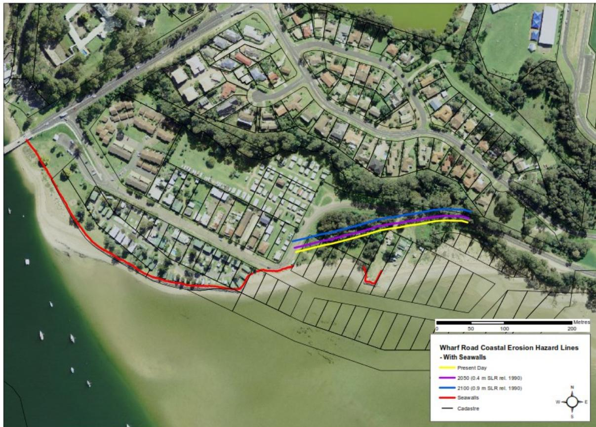
Note: Landward movement of the shoreline could be modified by the presence of bedrock. Hazard lines are located at seawall unless otherwise shown. The presence of an unapproved groyne has been ignored as ESC has requested it be removed.
