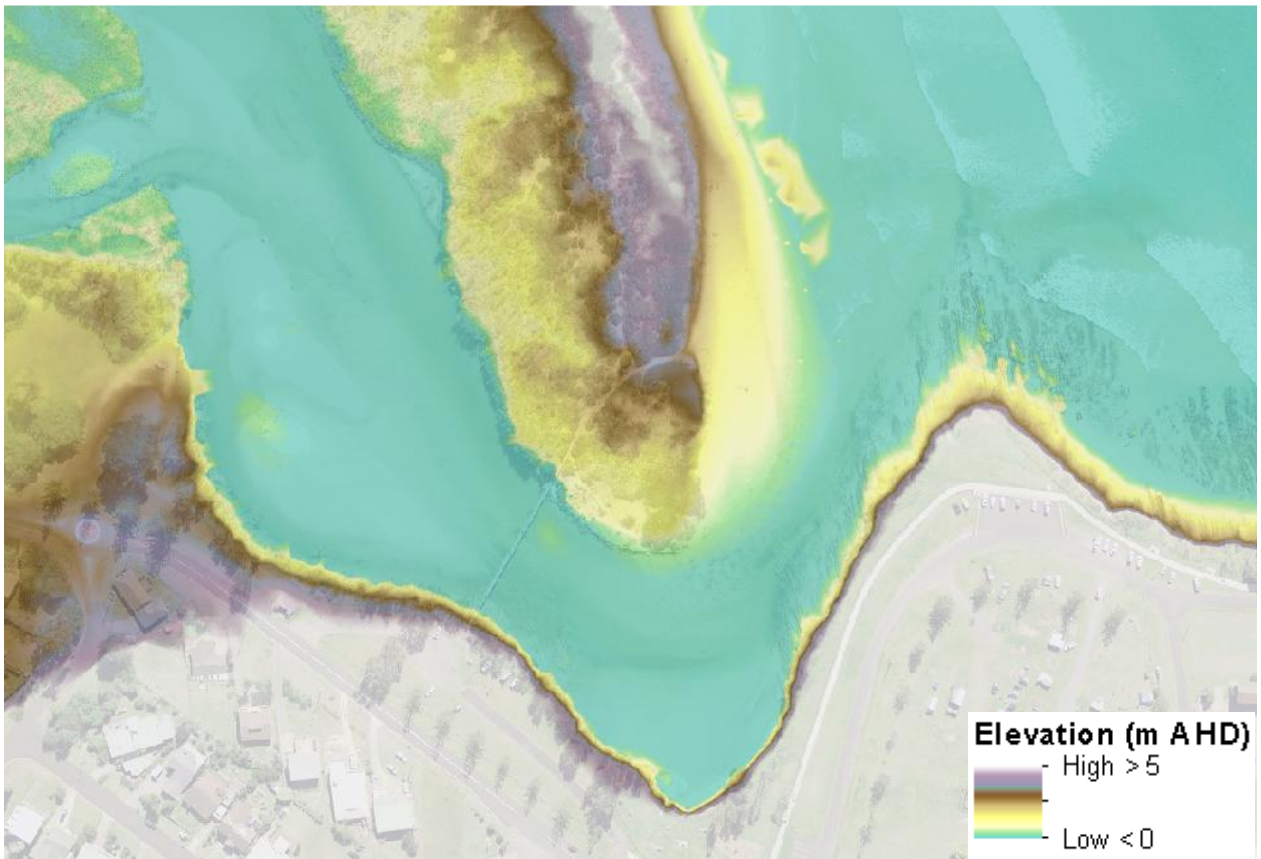
Diagram 12: Mummuga Lake ICOLL Entrance – DEM of 2012 LiDAR and 2013 bathymetric survey
