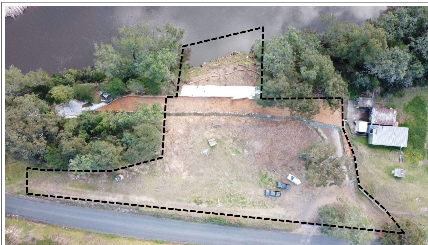
Figure 4-1 Overhead photo (looking down slope) of the TRIPS site post Stage 1 Vegetation Clearing works including indicative project boundary. The Tuross River borders the top of the photo and Eurobodalla Road borders the bottom of the photo. Clearance of vegetation on the riverbank face evident. Along riverbank slope, geotextile visibly installed on upper part of slope, with tree stumps remaining in place.
