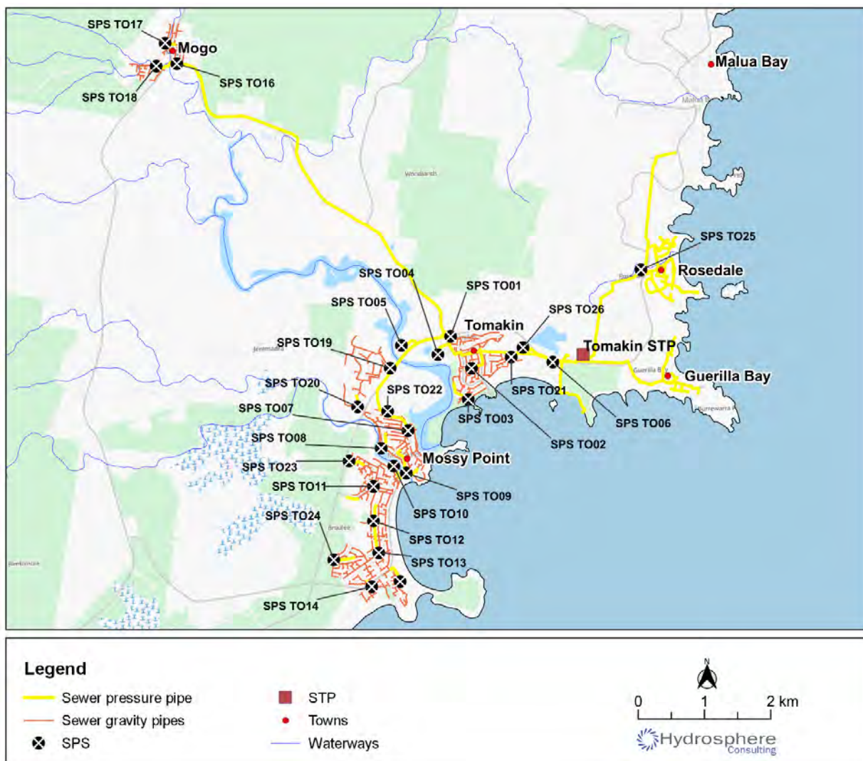
Figure 11: Tomakin sewerage system
