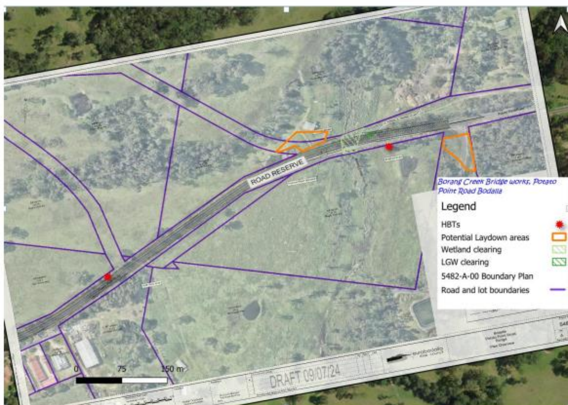
Figure 2. Work footprint for new bridge, culvert removal and road realignment/upgrade
