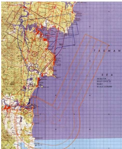
PANS-OPS surfaces for RNAV-Z approaches for RWY 18 / 36
