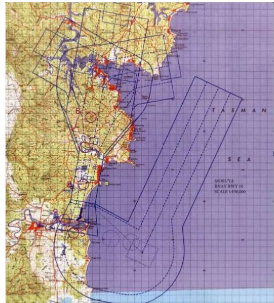
PANS-OPS surfaces for RNAV-Z approaches for RWY 18 / 36
