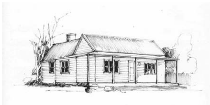
4. Weatherboard gable roofed cottage with partially enclosed verandah. Typical of Gundary area. Roof pitch around 35 degrees, minimum pitch (5 degrees) verandah. Ceiling height usually 3 metres. Verandah giving sun and weather protection to windows.
