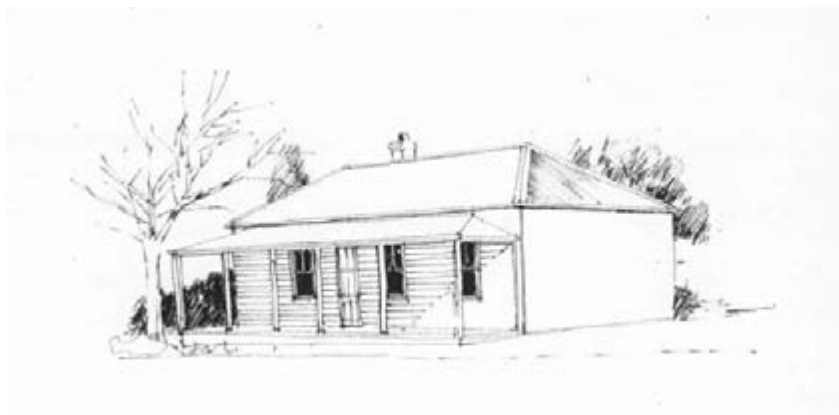
2. Classic weatherboard cottage with hipped roof and lower pitched hipped verandah to the street frontage. Vertically proportioned windows, slender hardwood posts with simple arched detailing. Corrugated steel roof. Ceiling height usually 3 metres.
