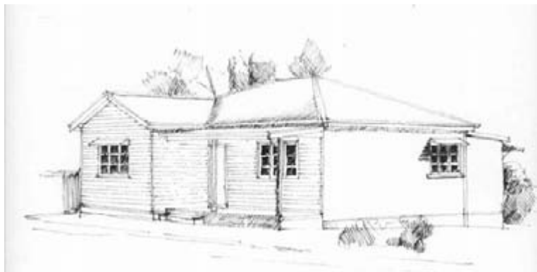
1. Weatherboard house with main hipped roof and gable to street frontage. Roof pitch usually 22 degrees, ceiling height over 2.7 metres. Use of simple low pitched verandah as entry transition space and weather protection. Corrugated steel roof and protective awnings over windows.
