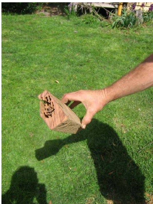
Evidence of termite damage to studs
