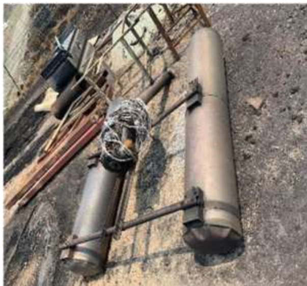
Two trailers and a pontoon mixer were destroyed at the sewerage treatment plant at Surf Beach. One was W&S Goodwin pump, the other was a tool trailer.
