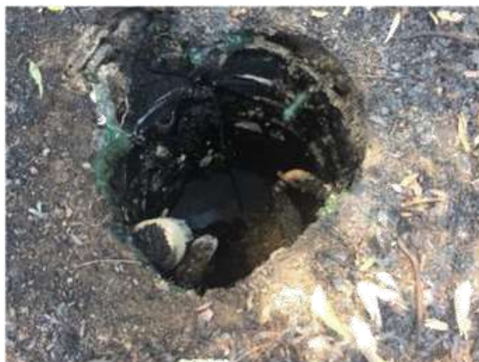
Example of destroyed pod & pump
