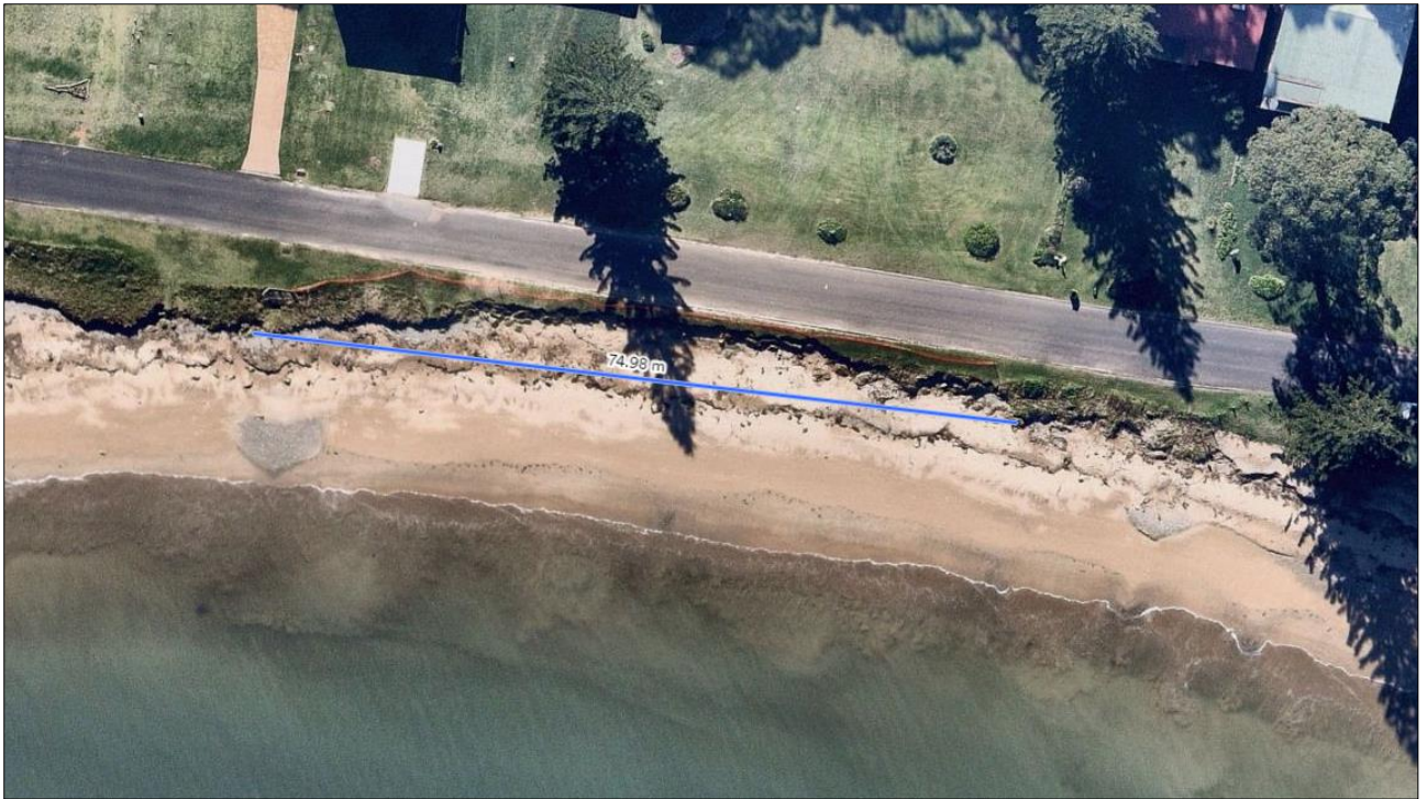
Figure 1: Image of Long Beach and Bay Road in respects to the eroded bank. The blue line illustrates the length and location of sandbags which will be placed along the site.
