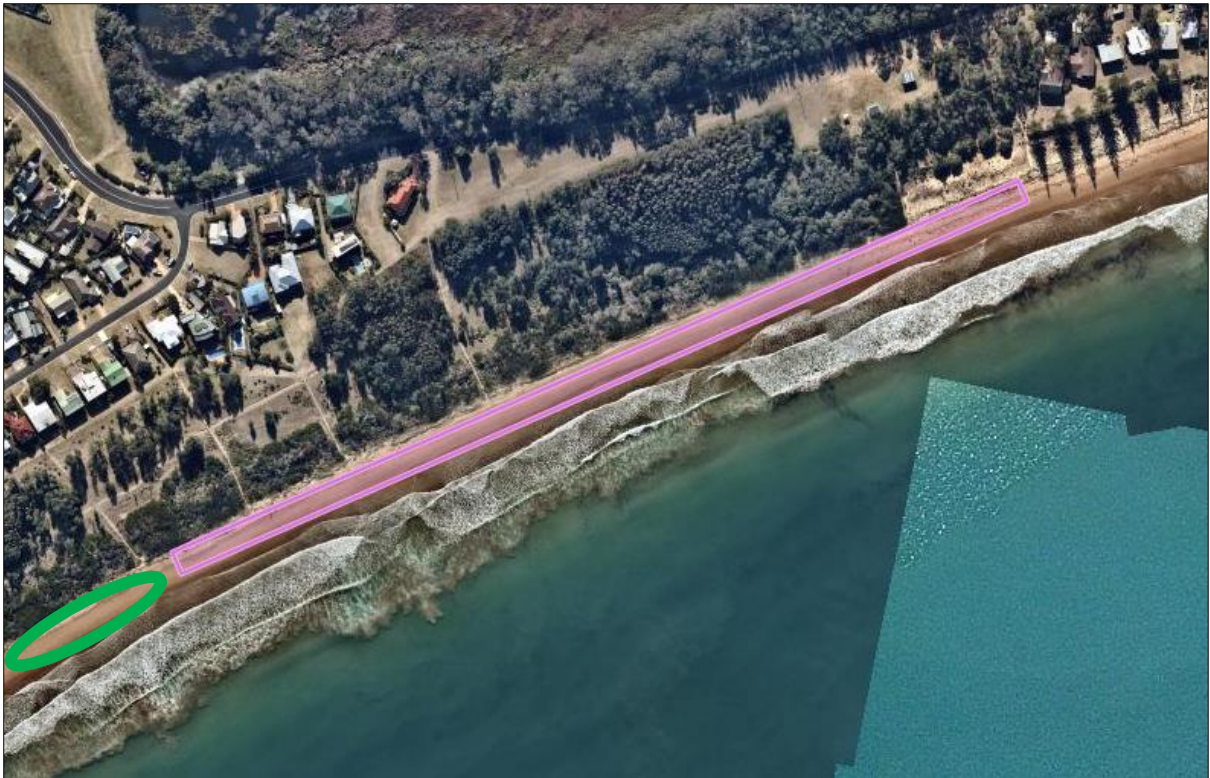
Figure 3: Indicative area where sand will be sourced. Approx. 2000m 3 (Pink area). Additional sand may be required outside of this area to the west (Green area).
