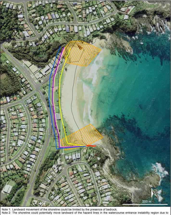
lowering of the beach profile from entrance scouring. Note 3: The shape of hazard lines not located at the seawall is hypothetical only and requires further detailed assessment beyond the scope of this study.
