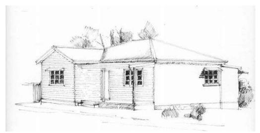
Weatherboard house with main hipped roof and gable to street frontage. Roof pitch usually 22 degrees, ceiling height over 2.7 metres. Use of simple low pitched verandah as entry transition space and weather protection. Corrugated steel roof and protective awnings over windows.
