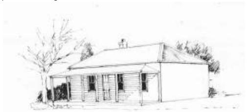
2. Classic weatherboard cottage with hipped roof and lower pitched hipped verandah to the street frontage. Vertically proportioned windows, slender hardwood posts with simple arrised detailing. Corrugated steel roof. Ceiling height usually 3 metres.
