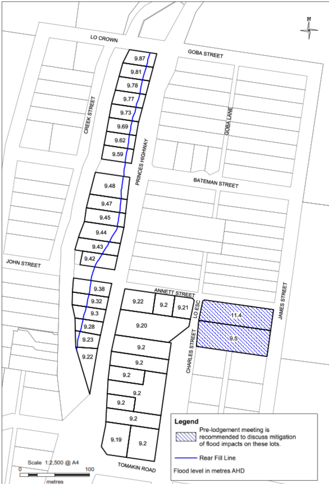
MAP 3 – Flood levels for a 1% AEP flood event. The flood planning level, in metres above the Australian Height Datum (AHD), is calculated by adding together the flood level shown in this map and the appropriate freeboard from part 6 of this Plan.
