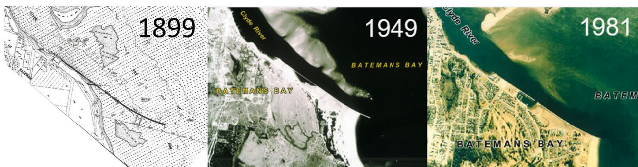
Figure 6-1 Rapid accretion of land behind the training wall at Corrigans Beach
